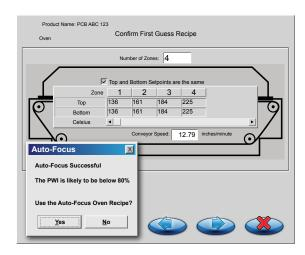
The KIC Auto-Focus and KIC Auto-Focus Power is simple, fast and easy to use, requiring minimal input or technical experience. Once the necessary criteria are provided, Auto-Focus goes to work and in seconds you are presented a suggested initial oven set up. The recipe is ranked using the Process Window Index (PWI), so you immediately know where it falls within your process specifications.
